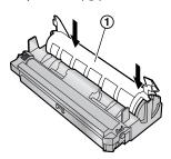
**9** Turn the two levers (1) on the toner cartridge firmly.
